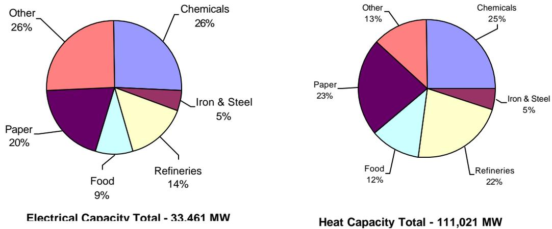
Industrial CHP electrical production was over 162,000 GWh and heat production was over 1.6 million TJ. As shown in Figure 5, 75% of the electrical production and 81% of the heat production in the industrial sector came from the same 5 industries:
