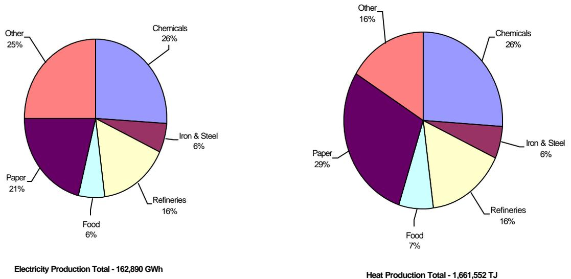
The distribution in use of the technologies for heat and electricity production (from all European CHP producers) is shown in Figures 6 and 7. Figure 6 shows the distribution by the amount of heat and electricity capacity in 1997. In summary:
